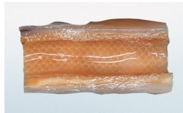
TISSUE INGROWTH and retention of smooth flow surface shown in an explant after 7 years in the femoro-popliteal position.
